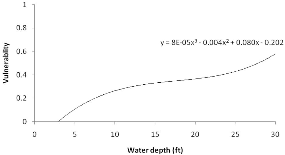
**Figure 12.** Vulnerability Function of Structure Type 1 with depth.
