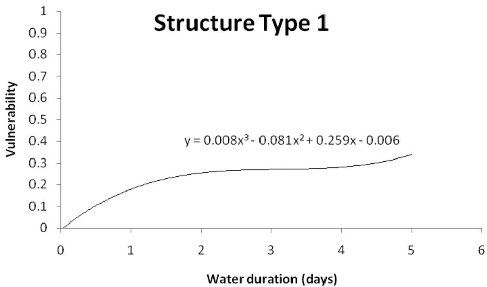
**Figure 13.** Vulnerability Function of Structure Type 1 with duration.
