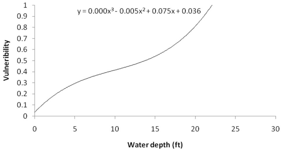
Figure 14. Vulnerability Function of Structure Type 2 with depth.
