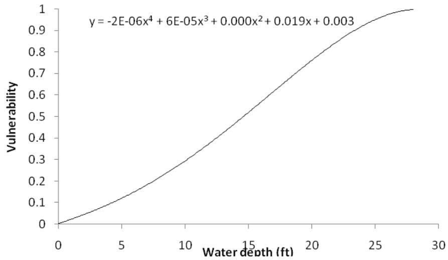
Figure 16. Vulnerability Function of Structure Type 3 with depth.
