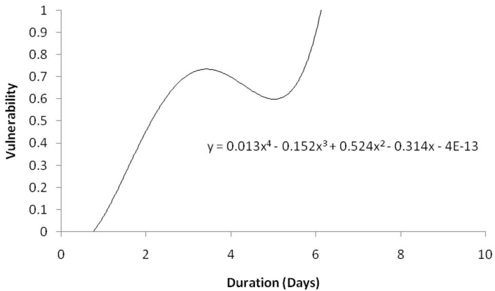
Figure 15. Vulnerability Function of Structure Type 2 with duration
