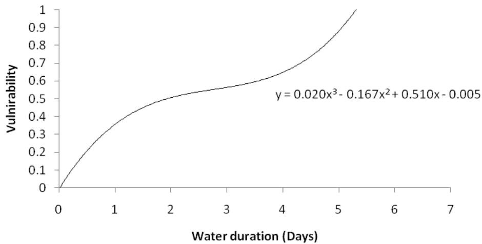
Figure 19. Vulnerability Function of Structure Type 4 with duration.
