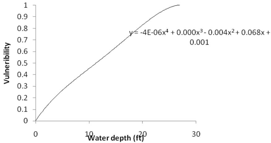
Figure 18. Vulnerability Function of Structure Type 4 with depth.
